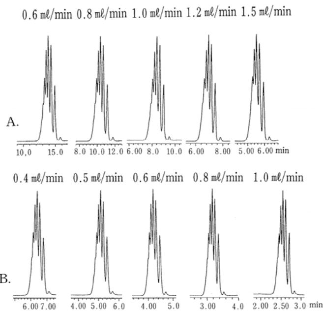
**Fig. 7** Flow rate dependence of separation of standard polystyrene in TSKgel SuperH2500 and G2500 H<sub>XL</sub> columns
