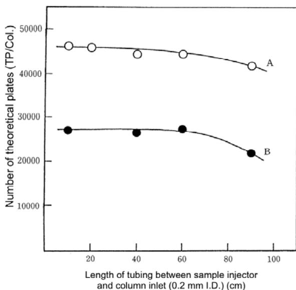
**Fig. 37** Relationship between number of theoretical plates and length of column inlet tubing in TSKgel SuperH2500
