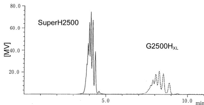
**Fig. 14** Comparison of peak heights of standard polystyrene (A-500) produced by TSKgel SuperH2500 and conventional columns (G2500H<sub>XL</sub>)
