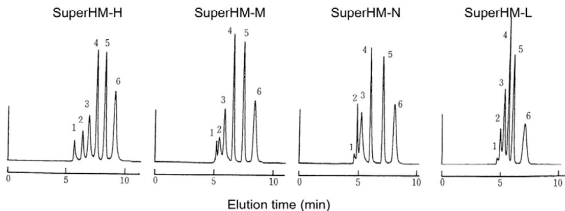
**Fig. 45** Comparison of separations of standard polystyrenes with the TSKgel SuperHM series (1)
