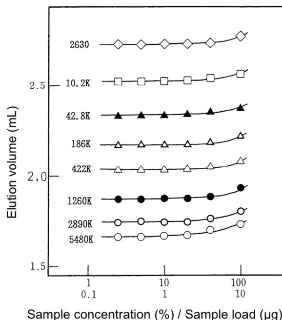
Fig. 23 Relationship between sample concentration (sample load) and elution volume for standard polystyrenes in TSKgel SuperHM-H
