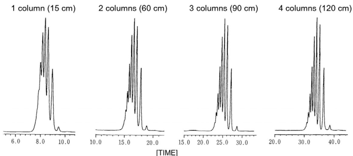
**Fig. 51** Dependence of separation of standard polystyrene (A-500) on column length in TSKgel G2500 H<sub>XL</sub>
