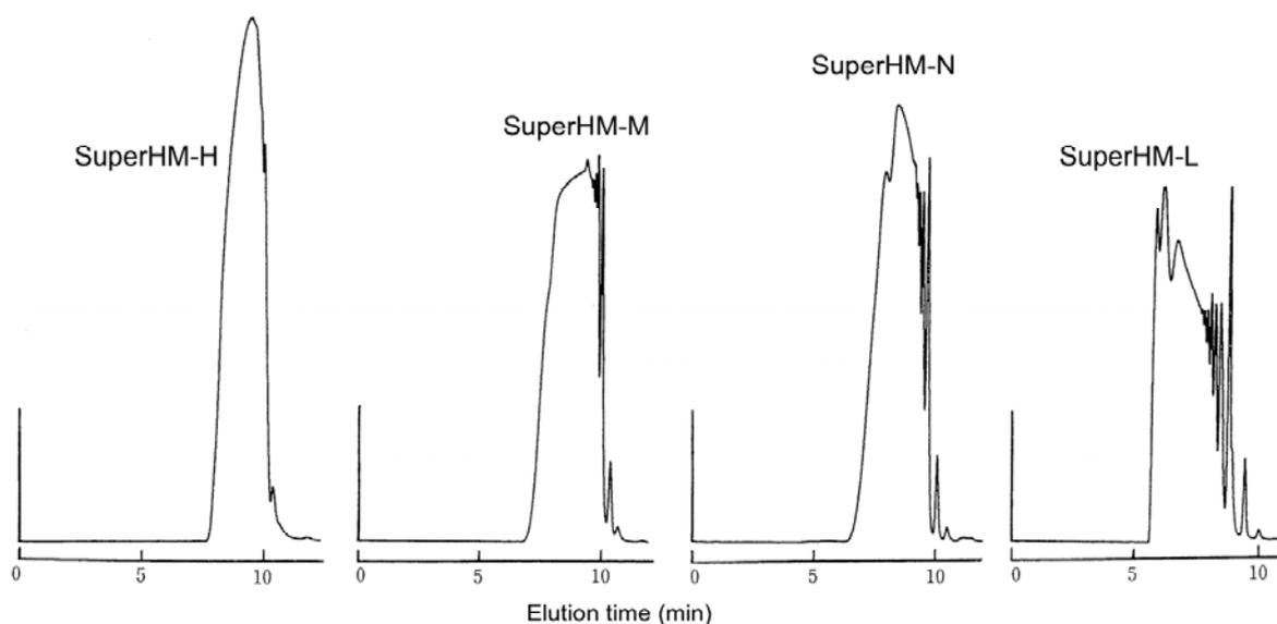
**Fig. 49** Comparison of separations of phenol resin with the TSKgel SuperHM series
