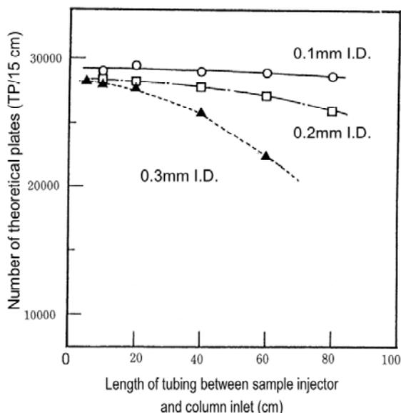
**Fig. 39** Relationship between number of theoretical plates and tubing inside diameter and length of column inlet tubing in TSKgel SuperH2500
