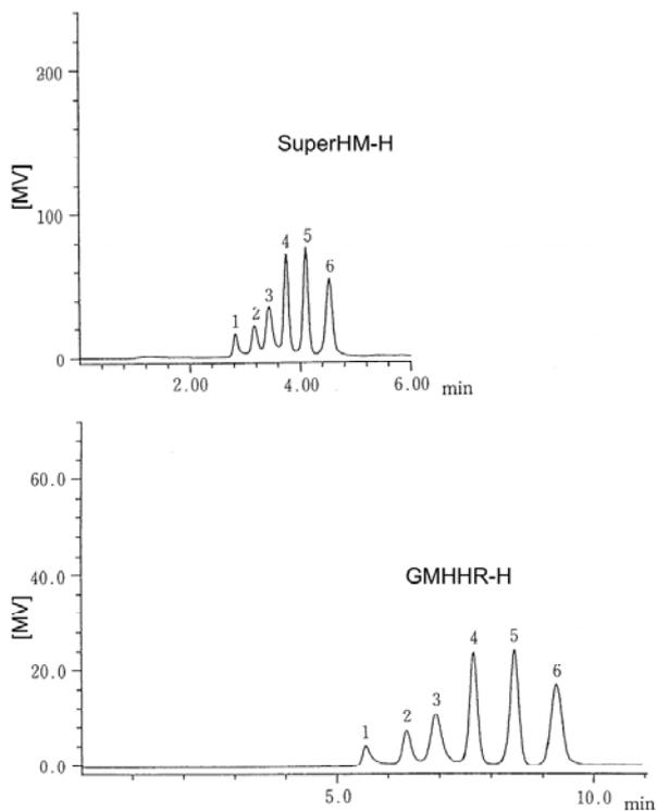
**Fig. 15** Separation of standard polystyrenes by TSKgel SuperHM-H and GMH<sub>HR</sub>-H
