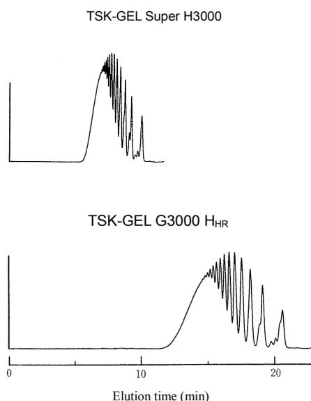
**Fig. 3 Separation of epoxy resin using TSKgel SuperH3000 and TSKgel G3000 H<sub>HR</sub> columns**
