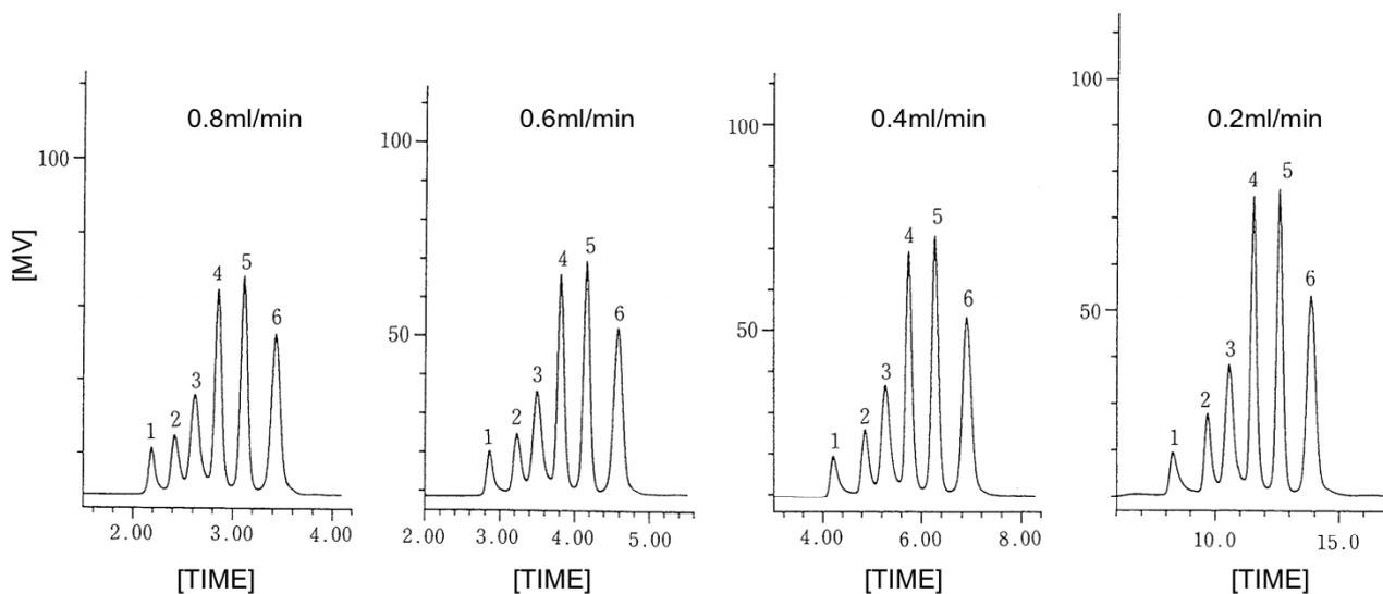
**Fig. 11** Flow rate dependence of separation of standard polystyrene in TSKgel SuperHM-H
