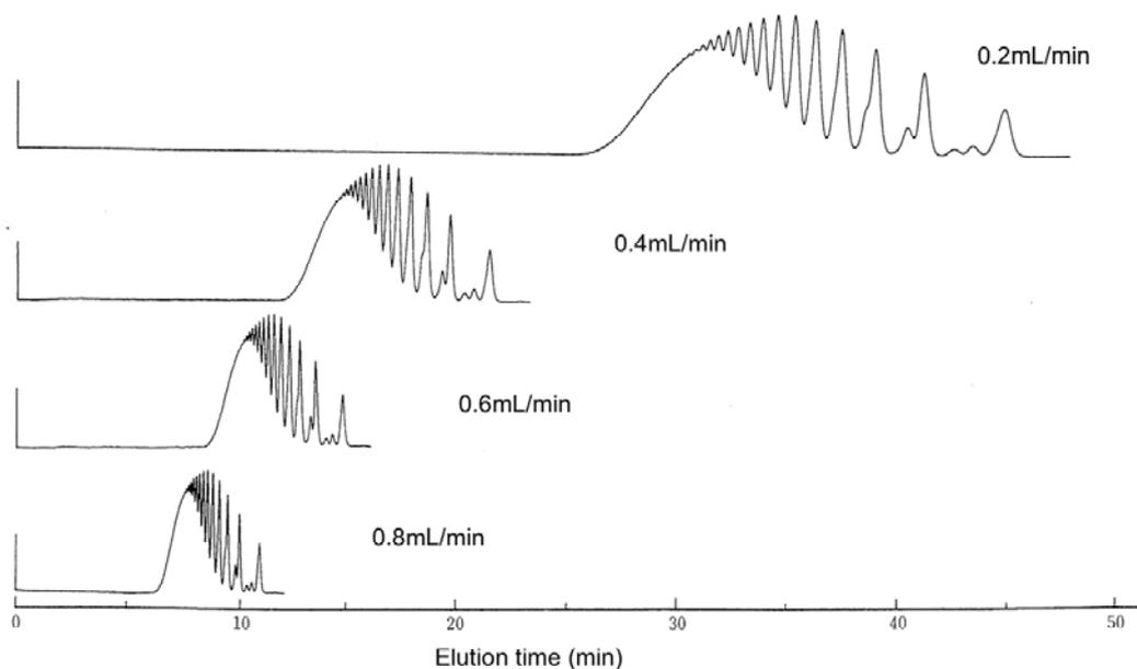
**Fig. 10** Flow rate dependence of separation of epoxy resin in SuperH columns
