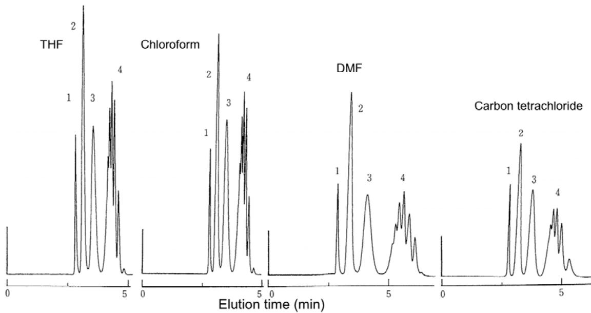
**Fig. 18** Separation of standard polystyrenes compared using various solvents with TSKgel SuperH2500
