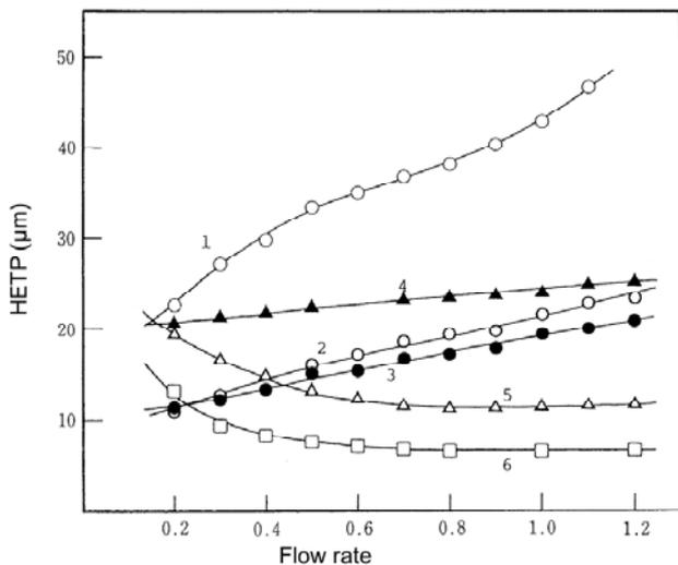
**Fig. 8** Relationship between HETP and flow rate at various molecular weights in TSKgel SuperHM-H
