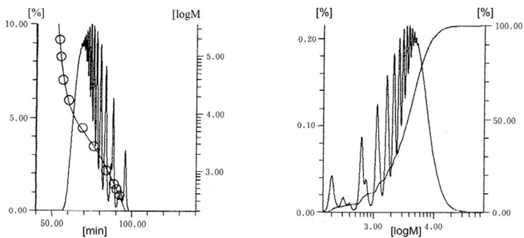
**Fig. 57** Separation of Epikote 1004 (E1004) using high speed GPC instrument (HLC-8120PC)
