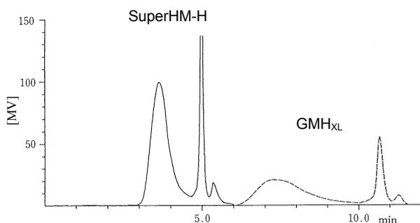
**Fig. 16** Comparison of commercial polystyrene peak heights produced by TSKgel SuperHM-H and conventional columns
