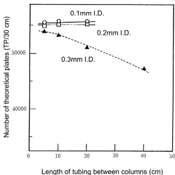
**Fig. 40** Relationship between number of theoretical plates and inside diameter of tubing and length of connecting tubing between columns in TSKgel SuperH2500
