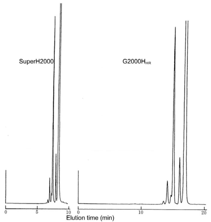
**Fig. 54** Comparison of separation of epoxy resin in TSKgel SuperH2000 and G2000 H<sub>HR</sub> columns
