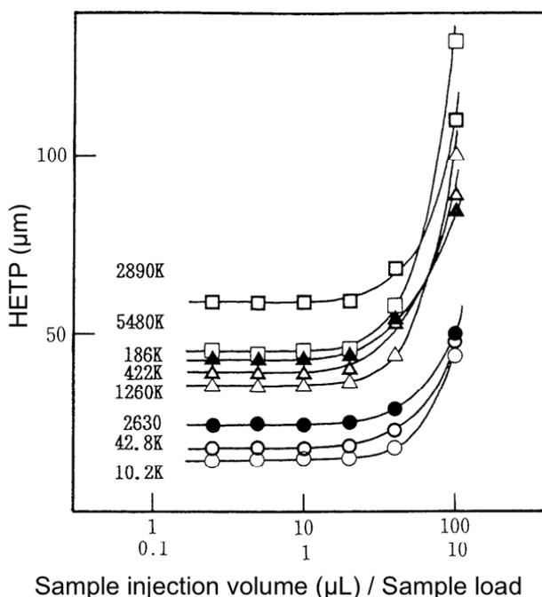
Fig. 22 Relationship between sample injection volume (sample load) and HETP for standard polystyrenes in TSKgel SuperHM-H
