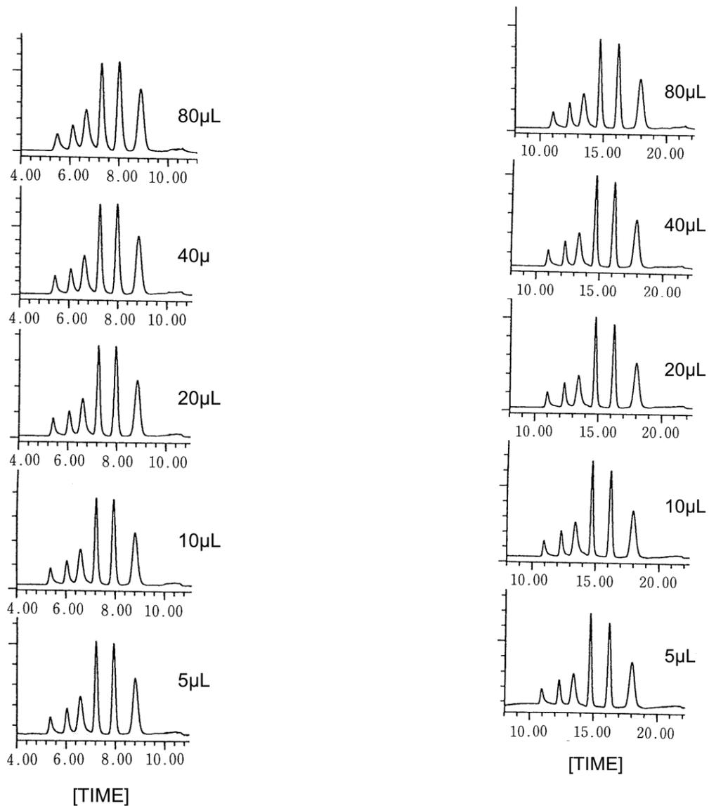
**Fig. 26** Effect of sample load on separation of standard polystyrene using TSKgel SuperHM-H
