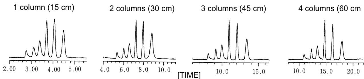
**Fig. 52** Dependence of separation of standard polystyrene on column length in TSKgel SuperHM-H
