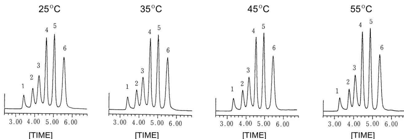
**Fig. 34** Temperature dependence of separation of standard polystyrene in TSKgel SuperHM-H
