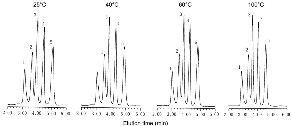
**Fig. 56** Temperature dependence of separation of standard polystyrene with the TSKgel SuperHM-H
