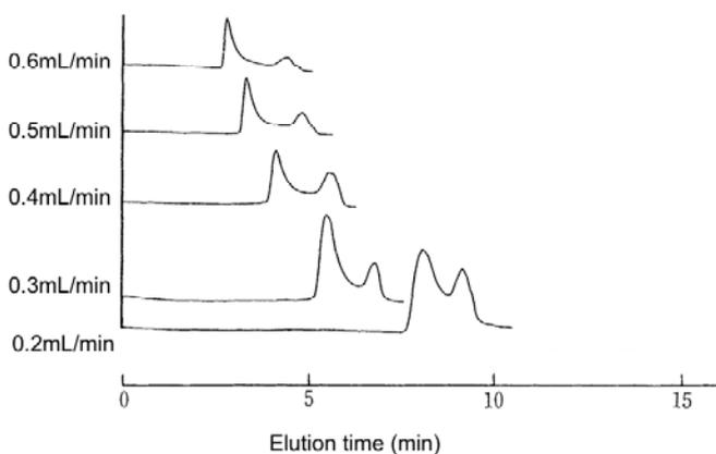
Fig. 28 Dependence of shear degradation on flow rate in TSKgel SuperHM-H
