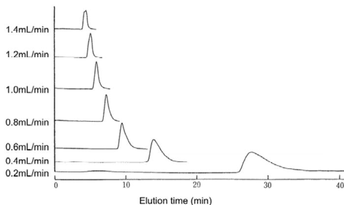
Fig. 29 Dependence of shear degradation on flow rate in TSKgel GMH<sub>HR</sub>-H (S)
