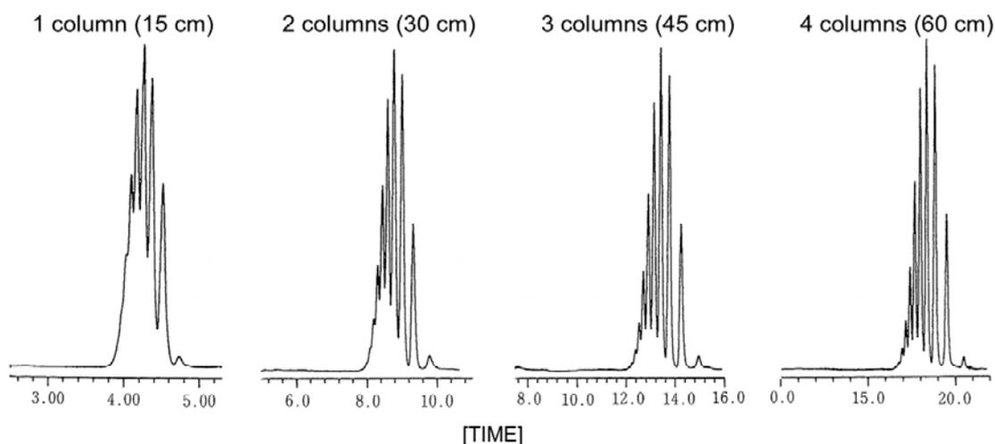
**Fig. 50** Dependence of separation of standard polystyrene (A-500) on column length in TSKgel SuperH2500
