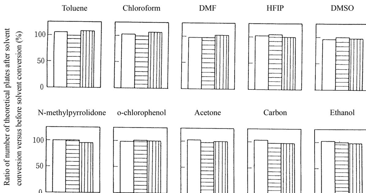
**Fig. 17** Solvent compatibility of TSKgel SuperH Series
