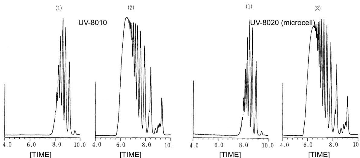
**Fig. 36** Dependence of separation performance on band spreading in detector in TSKgel SuperH2500
