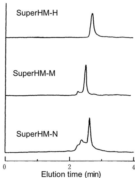
Fig. 32 Comparison of shear degradation of standard polystyrene F-850 using the SuperHM series
