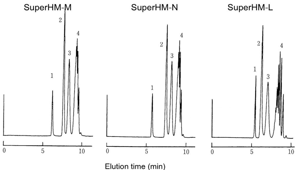
**Fig. 46** Comparison of separations of standard polystyrenes with the TSKgel SuperHM series (2)
