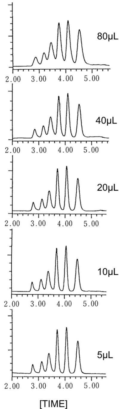
**Fig. 25** Effect of sample load on separation of standard polystyrene using TSKgel SuperHM-H
