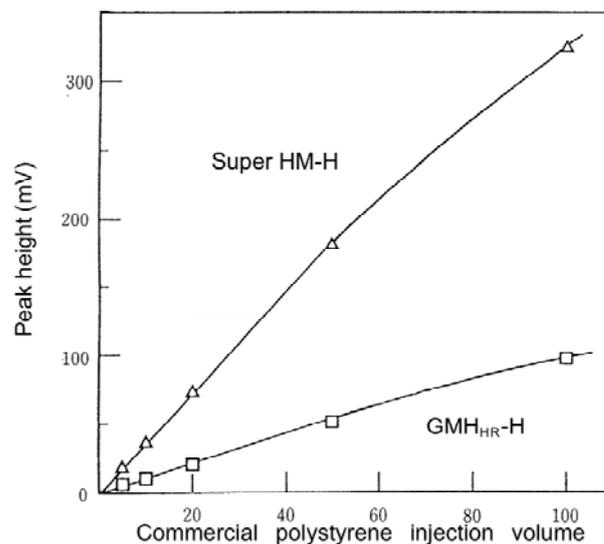
**Fig. 13** Relationship between peak height and injection volume of polystyrene using TSKgel SuperHM-H and GMH<sub>HR</sub> columns
