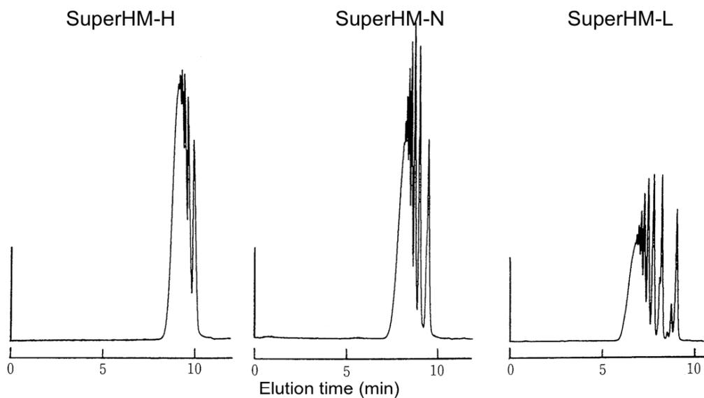
**Fig. 47** Comparison of separations of epoxy resin with the TSKgel SuperHM series (1)
