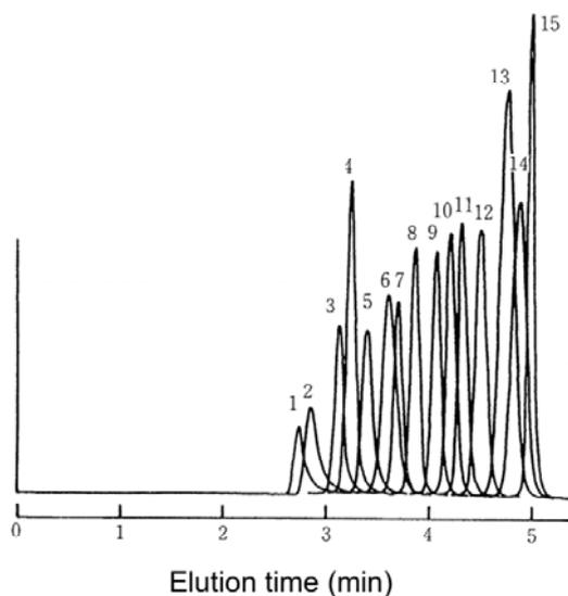
**Fig. 44** Elution curve of standard polystyrene using TSKgel SuperHM-H
