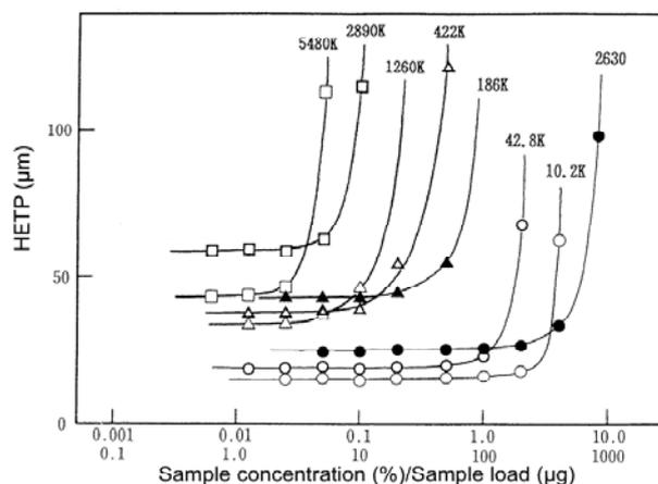
**Fig. 20** Relationship between sample concentration (sample load) and HETP for standard polystyrenes in TSKgel SuperHM-H
