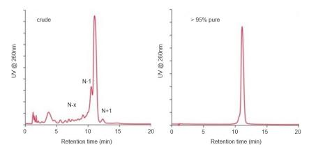
Fig. 3: AIEX analysis of crude and purified 20mer oligonucleotide on TSKgel DNA-STAT
