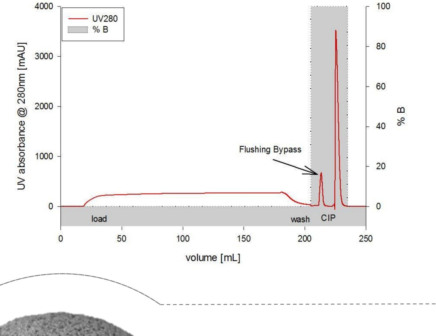
40 CV of the aggregated Protein A eluate were loaded on the column at 1 residence time. min Monomer flows through column during the loading. No elution of the bound aggregate was performed. Area of CIPpeak indicates the amount of bound aggregate.
