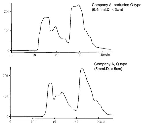
**Figure-5** Comparison of separation with various ion exchangers under large sample load
