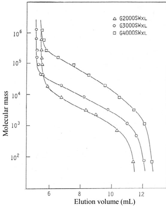
**Figure 1 Calibration curves produced with PEG**
