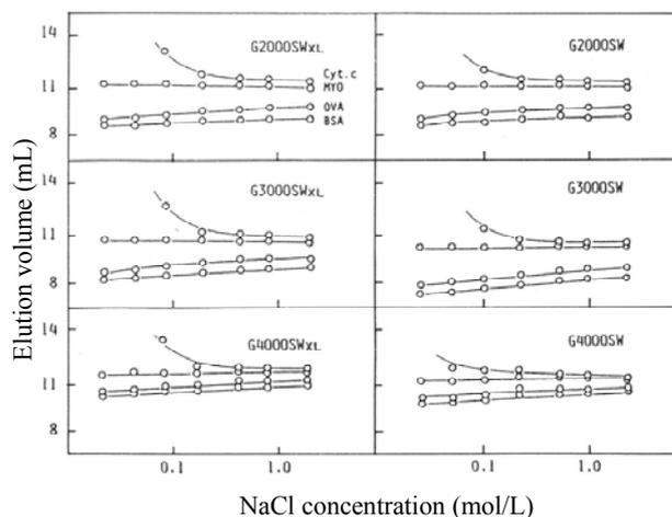
**Figure 8** Dependence of elution volume on salt concentration
