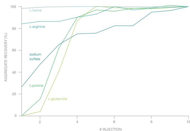
➤ **AGGREGATE RECOVERY ON NEW TSKgel UltraSW AGGREGATE COLUMNS**
