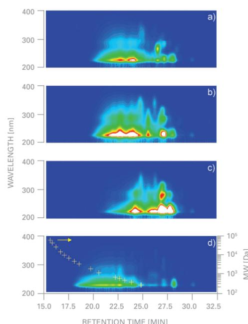
➤ GPC ANALYSIS OF THERMALLY TREATED LIGNIN
