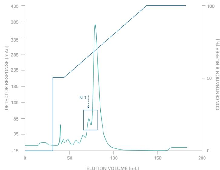
➤ PURIFICATION OF OLIGONUCLEOTIDES ON TSKgel SuperQ-5PW (20)
